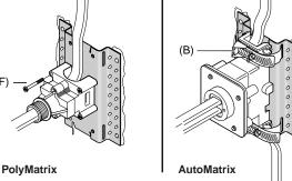
· For AutoMatrix kits, fasten stand to plate two pipe straps (B).
