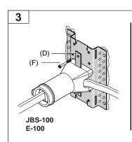
• For JBS-100 and E-100 connections, fasten stand to plate using connection bar (D) and two screws (F).
