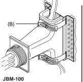
• For JBM-100 and T-100 connections, fasten stand to plate using two pipe straps (B).
